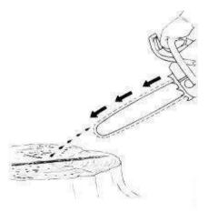
8.1 The chain oil flow can be altered by inserting a screwdriver in to the hole on the underside of the chain saw and adjusting the oil flow according to your work conditions.
