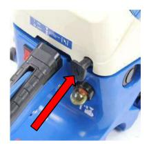
Disengage the chain brake by pulling the handle backwards, away from the chainsaw blade. DO NOT attempt to rev the engine or use the machine with the chain brake engaged (in the forward position).
