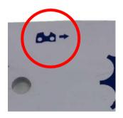
3.6 Adjust the position of the chain tensioner stud on the chain cover moving it back towards the lower adjustment hole on the guide bar. (5).
