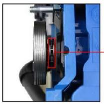
Ensure the chain slots onto the clutch sprocket, instead of either side.
