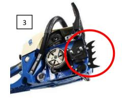
3.5 Install the guide bar over the 2 studs and whilst wearing thick protective gloves, place the chain round the rear sprocket and the guide bar (4).
