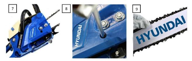
Tighten the chain cover nuts securely with the bar tip held up (12~15Nm).
